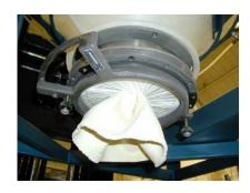
A useful option to use in conjunction with the H type Iris Valve is a Liner. A Liner is simply a tube of flexible material, which passes through the valve, which is constricted (or throttled) by a closing diaphragm.
